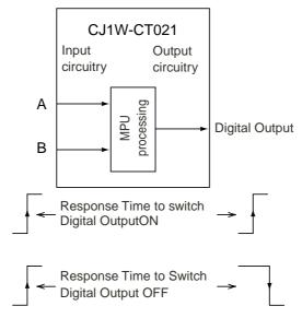
The Response Time can vary between 0.1 and 0.5 milliseconds, but is guaranteed to be less than 0.5 milliseconds. The following factors cause the Response Time to fluctuate:
