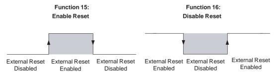
To reset a Counter by the function 05 or function 06, it is necessary for external resets to be in the enabled state and for Reset Enable to be set to 1. For details on Counter resets, refer to 3-6 Reset Counter.
