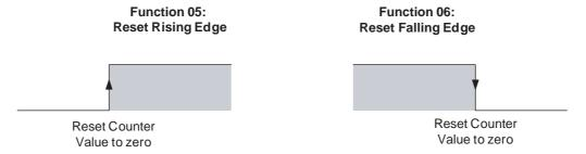
To reset a Counter by the Function 05 or 06, it is necessary to set the following variable Reset Enable to 1.
