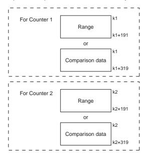
k1, k2: Start address for comparison data area for Counter 1 and Counter 2. Specify the allocated address from Memory Address screen in Edit Special Unit Settings of Sysmac Studio.
