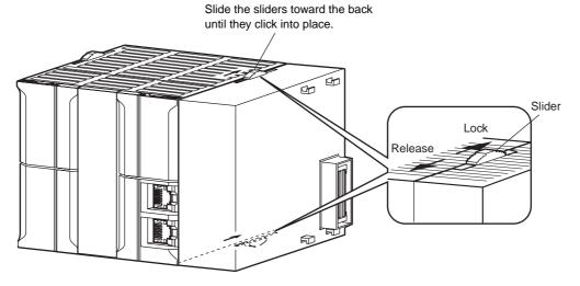
3 Attach an End Plate to the Unit on the right end of the Rack.
