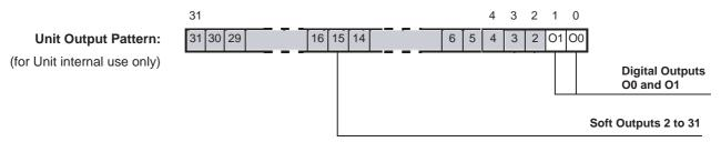
Digital Outputs 0 and 1 correspond with the Digital Outputs O0 and O1.
