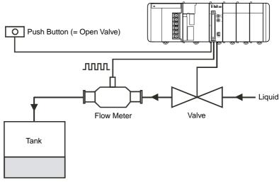
This is an application that puts a certain amount of liquid in the tank. This application measures the flow of incoming liquid with a flow meter and controls the liquid injection valve.
