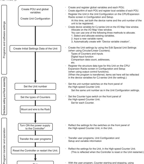
At this time, an I/O Setting Check Error occurs when there is a Unit Configuration in the CPU Unit which does not match the actual Unit Configuration. In this case, reset the Controller in Reset the Controller or restart the Unit process to cancel the error.
