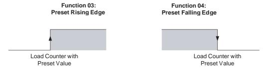
This Unit has device variables for CJ-series Unit (for output) to store preset values for Counters. To change a preset value, set a preset value in this variable.
