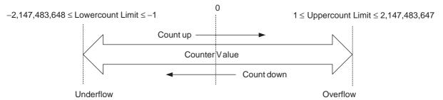
If a Counter Value exceeds the Upper Count Limit, an overflow is set in the device variable for CJseries Units; if a Counter Value is below the Lower Count Limit, an underflow is set.
